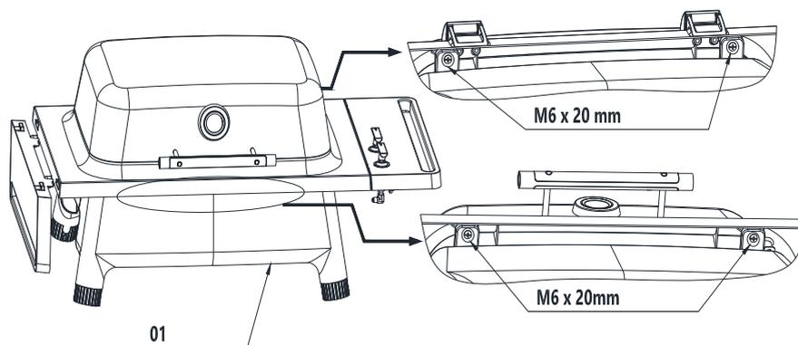
Angle the assembly slightly to the back and remove both M6x20mm screws, then do the same at the front, supporting the parts so they don't drop. Keep all of the fasteners for later use. Removable stickers at the front and rear will mark the positions of these screws. Remove the hood and barbecue chassis assembly from the stand top and place on the ground.
